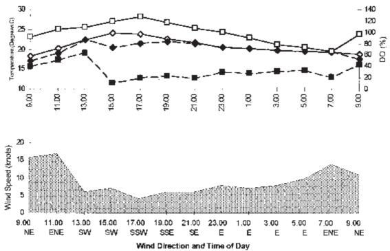
**Figure 1.** Temperature (°C) and DO saturation (%) readings for the top and bottom of the water column at sites 1, 2 and 3, and windspeed and direction over the 24 hour study period from 20 to 21 March 1993. Temperature top  $\diamond$ , temperature bottom  $\blacklozenge$ , DO top  $\Box$ , DO bottom  $\blacksquare$ .
