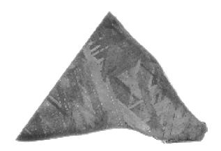
**Figure 5.** Cut, polished and acid treated slice of the Haig iron meteorite showing the Widmanstätten pattern characteristic of this group of irons (sawn edge measures 8 cm).
