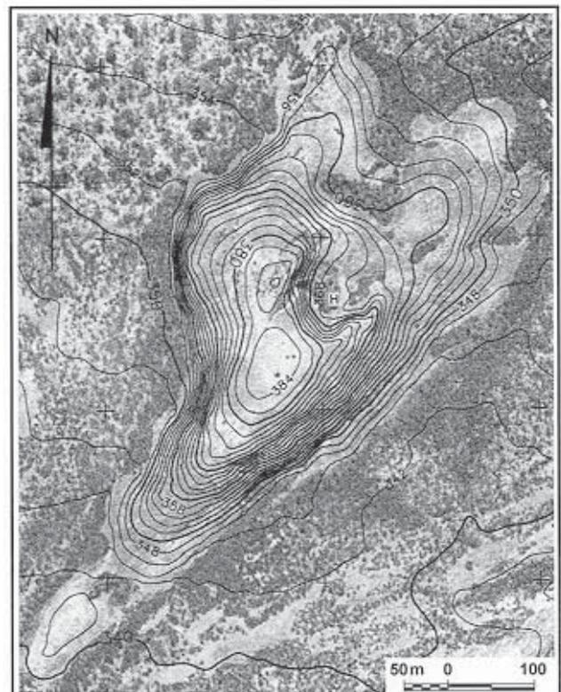
**Figure 11.** Bank Rock: topography, indicated by two metre form lines, superimposed on vertical aerial photograph. Note that the crosses are part of the form-line plot. (Extract from photo-map drawn by McMullen, Nolan and Partners Surveyors, WA).
