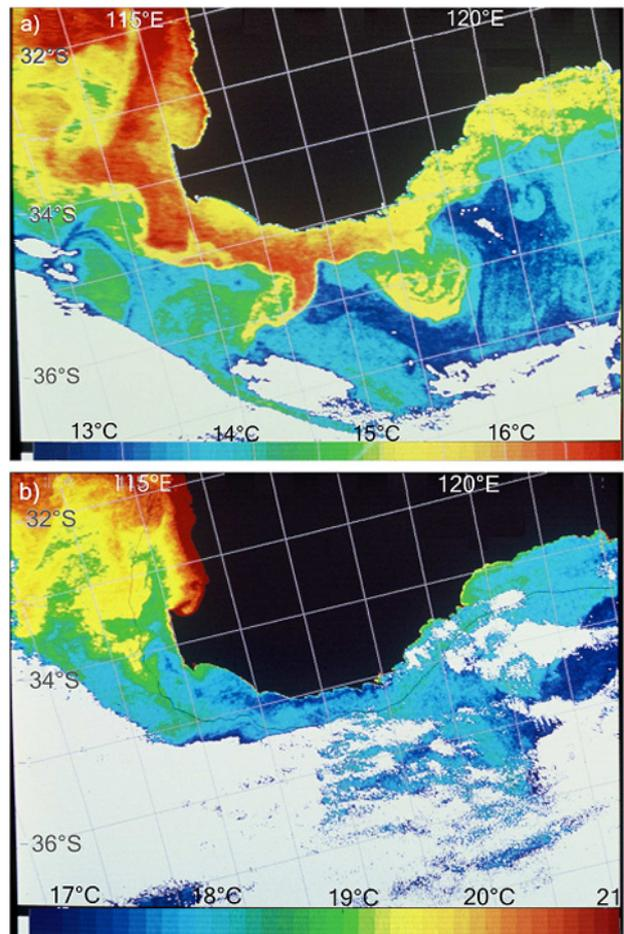
**Figure 2.** Satellite sea-surface temperature images from south of Western Australia: a) 18 November 1986; and b) 6 March 1987. The temperature scale is at the bottom of each image; clouds are white; a black mask has been put over the land; and there is a 1 × 1° latitude–longitude grid. Data from NOAA 9 satellite received by CSIRO in Hobart. 2b is from Cresswell & Peterson (1993, plate 1c).
