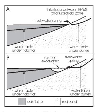
Figure 4. Mechanisms by which freshwater discharge from the red sand dunes forms springs and wetland zones along the contact of Mowanjum Sand and Sandfire Calcilutite. A. The Sandfire Calcilutite impedes freshwater discharge and forms freshwater springs. B. The Sandfire Calcilutite impedes freshwater discharge forming a freshwater spring which solution-excavates a wetland basin.
