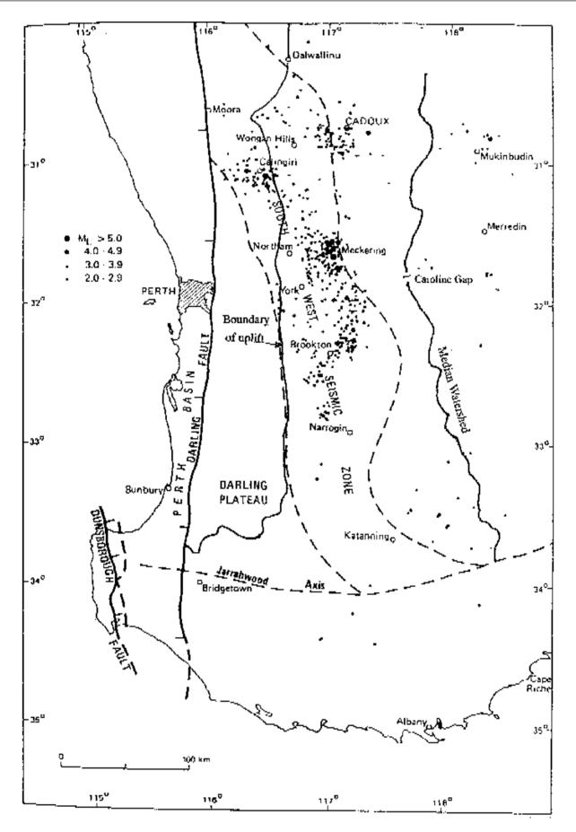
Figure 6. The South-West Seismic Zone (after Lewis et al. 1981) contrasted with the Median Watershed and the Darling Plateau uplift.
