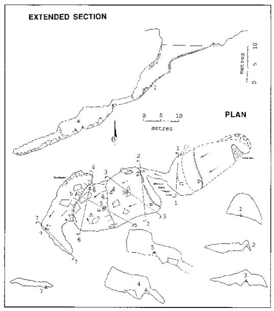
**Figure 1.** Plan and extended section of Bundera Sinkhole. The floor is mainly boulder breakdown. Algal/bacterial growth is depicted by the fringes near the top of the section. The lines vvvv denote the limit of ambient daylight and the limits of daylight sighting under optimal (first-dive) conditions. The numbered lines in the plan denote the location of the cross sections below numbered 1 to 7. Surveyed by A Poole and D Warren, 24-26 May 1995 to Grade BCRA Standard 3C.
