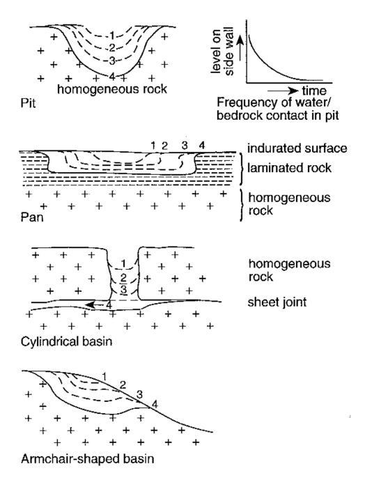
Figure 7. Schematic development of pits, pans, cylindrical gnammas and armchair shaped rock basins (After Twidale 1982).
