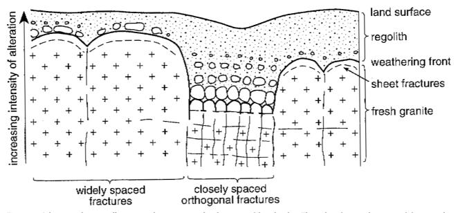
**Figure 2**. Schematic diagram illustrating the two-stage development of bornhardts. The subsurface exploitation of fractures by weathering is followed by the erosion of the regolith and the exposure of the weathering front. A similar two-stage or etch explanation of boulders is also illustrated (after Twidale 1982).
