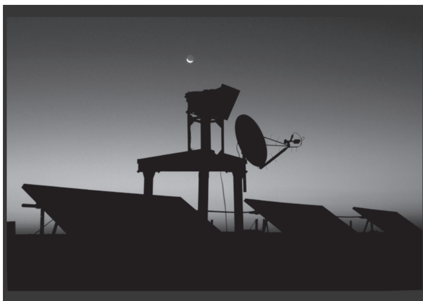
Figure 7 A fireball observatory of the Australian Desert Fireball Network on the Nullarbor in Western Australia, with solar power and satellite link (Courtesy of Geoff Deacon).
