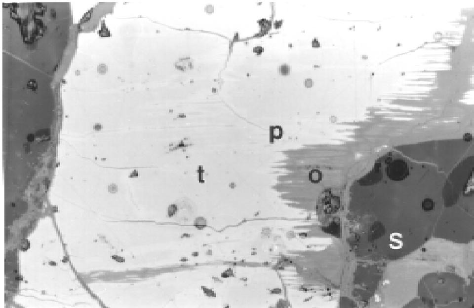
**Figure 4.** Extensively weathered particle of troilite (t) with dark grey iron oxides (o) surrounded by silicates (s). Weathering of troilite has progressed along (0001) parting planes and there is incipient development of pentlandite (p). Field of view 0.2 mm.
