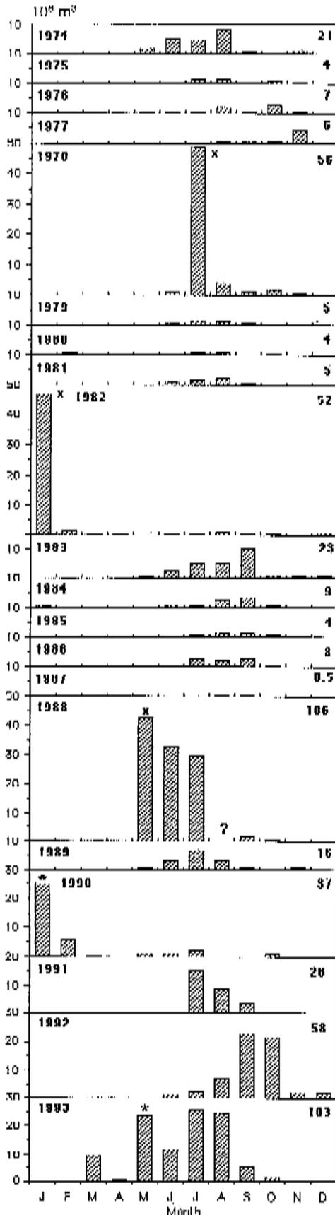
Figure 6. Monthly and annual flow (10<sup>6</sup> m<sup>3</sup>) in the Pallinup River, from gauged catchment 602001 (3655 km<sup>2</sup>). Data from the Water and Rivers Commission, Perth.
