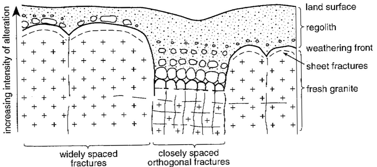
**Figure 2.** Schematic diagram illustrating the two-stage development of bornhardts. The subsurface exploitation of fractures by weathering is followed by the erosion of the regolith and the exposure of the weathering front. A similar two-stage or etch explanation of boulders is also illustrated (after Twidale 1982).
