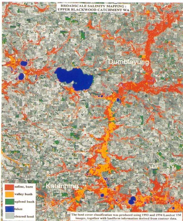
**Plate 4.** A typical application of Landsat-TM is to map areas of salinisation by classification. This example is an area of the grain belt of Western Australia, 200 km south east of Perth covering an area of about 2,000 km<sup>2</sup>. The technique uses two successive Landsat-TM images during the winter period of crop growth and digital elevation data to classify areas affected by salinity.
