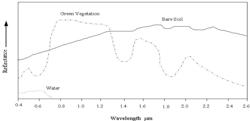
**Figure 4.** Typical reflectance spectra of dense green vegetation, soil and pure water (Modified from Legg 1992)
