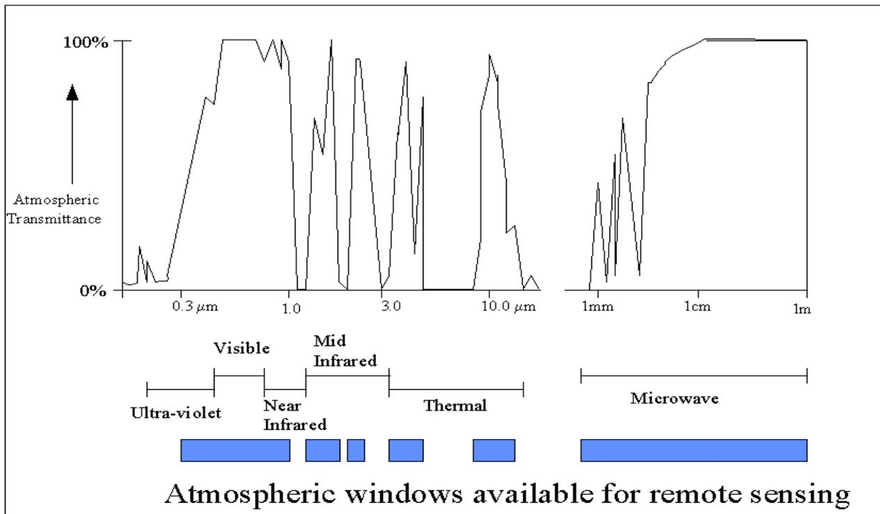
Figure 3. Portions of the electromagnetic spectrum used for remote sensing, showing the main subdivisions and atmospheric windows (modified from Legg 1992).
