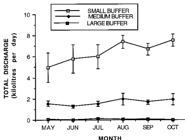
Figure 3. Mean ( $\pm$ SEM) surface runoff (in kilolitres per day) from the three different-sized buffer zones during each sampling occasion. Sampling sizes for the small and medium buffers,  $n = 3$  on each occasion. A single sample was taken from the large buffer zones (site 8).
